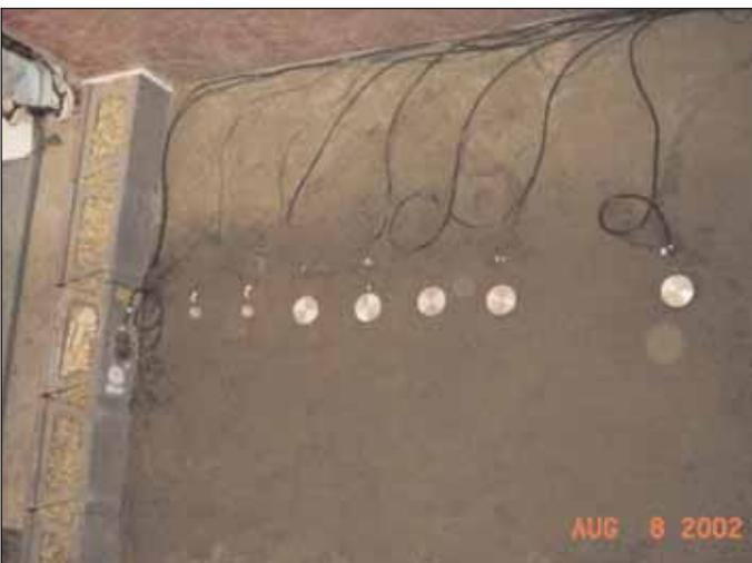
Load Transducers for Measuring Vertical Earth Pressure
