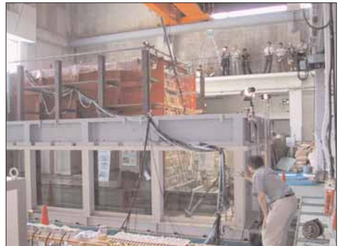
Steel Container for Wall Construction
