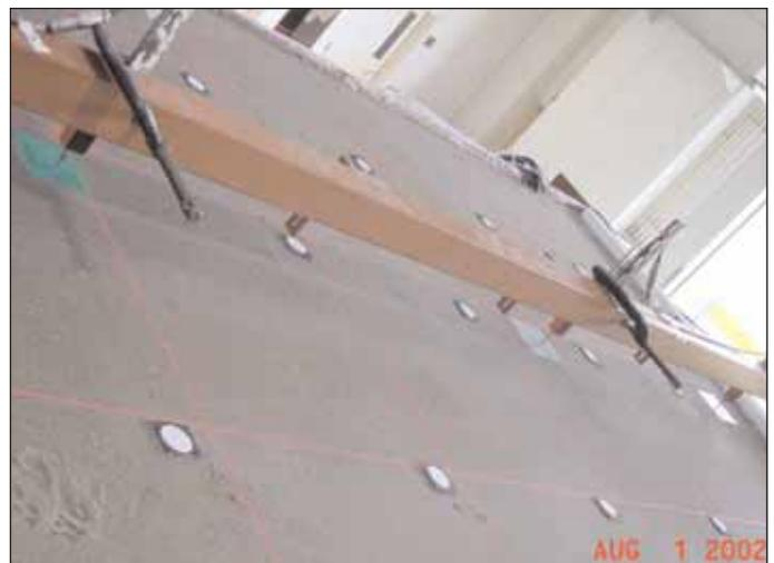
LVDT and Markers on the Backfill Surface
