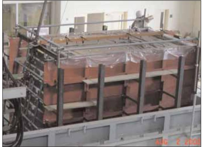
General Appearance of Test Wall after Second Shaking Load Application
